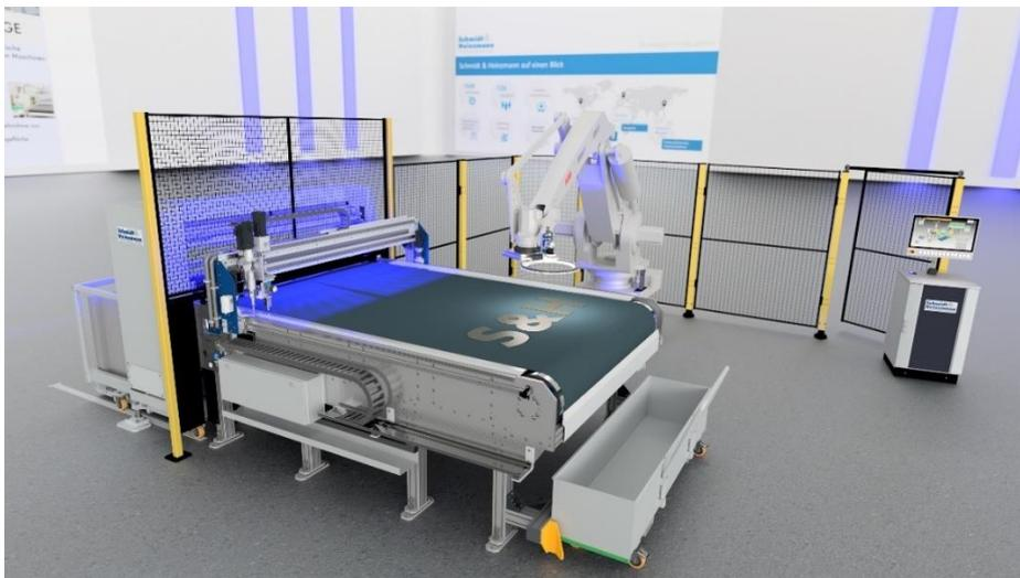
*Kamerasystem an Cutting & Stacking Anlage*
