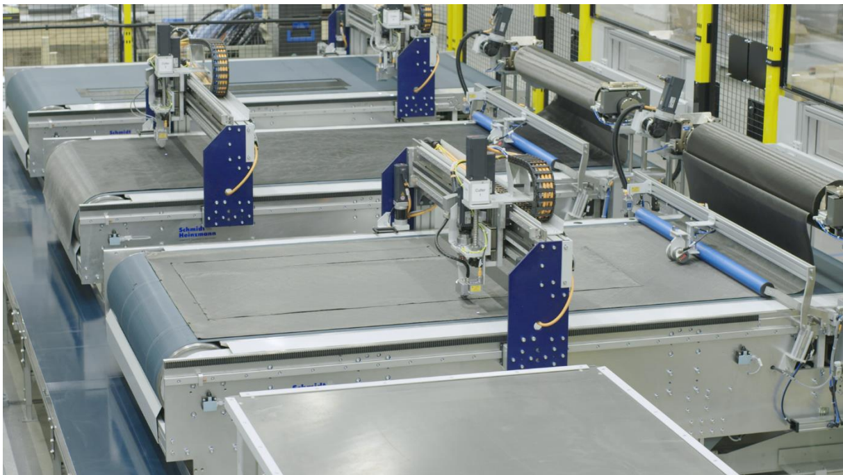
Cutting & Stacking Cell for dry fibers with several cutting tables of the model "AutoCut".
