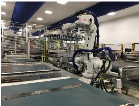
„ThinKing December“ Cutting & Stacking cell for processing of dry fibers Bild: Schmidt & Heinzmann GmbH & Co. KG
