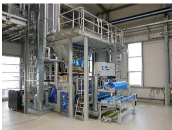
„JEC Award“ finalist – Machine for production of semi-finished SMC material "Cube" Bild: Schmidt & Heinzmann GmbH & Co. KG
