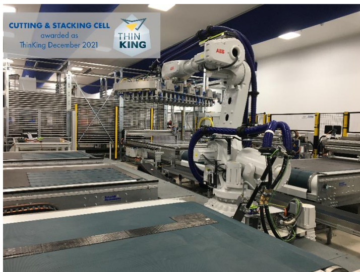
6 Cutting tables and one central robot produce 16 stacks in parallel Bild: Schmidt & Heinzmann GmbH & Co. KG
