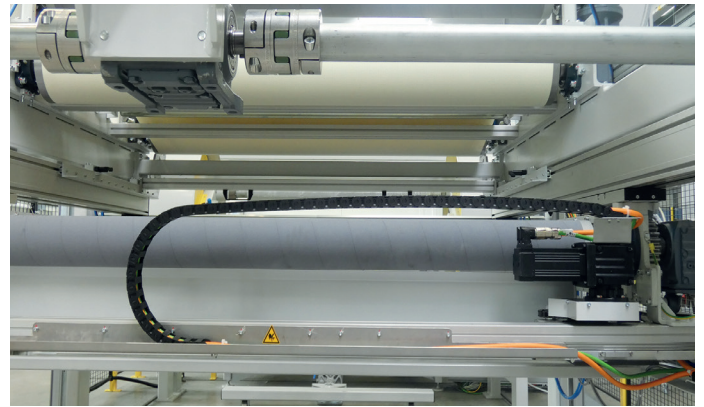
The material buffer allows continuous production without machine stop during automated ejection of full material boxes.
