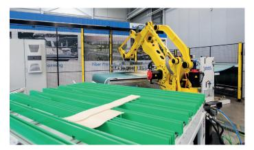
Automated weighing of the cuts and automated correction of the following cuts, if necessary, ensures to keep the total weight of the stack
