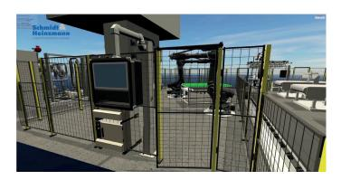
Especially when space is limited and when integrating into existing production environments, it is often very useful to plan the production cell via virtual reality.
