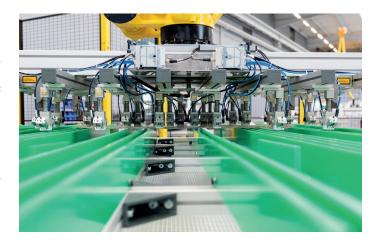
A robot with stacking gripper reliably and quickly stacks the cuts to their place.
